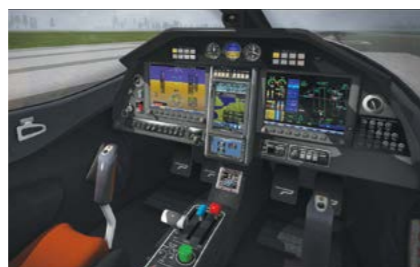
The haptic interface for the aircraft's propulsion lever helps the pilot communicate more easily with the powertrain.
